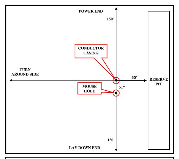
**Note:** <u>All</u> measurements are from the center of the conductor casing. The mouse hole is 51" from the center of the conductor casing  $w/0^{\circ}$  slope (angle). This rig has a top drive so the mouse hole should be a minimum of 75' deep (from ground level) with casing or liner with a minimum ID of 10". The reserve pit is a minimum of 50' from the center of conductor casing.
