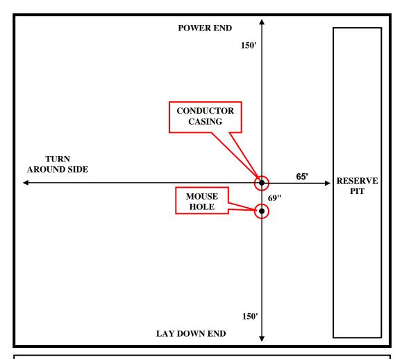
**Note:** <u>All</u> measurements are from the center of the conductor casing. The mouse hole is 69" from the center of the conductor casing w/0° slope (angle). This rig has a top drive so the mouse hole should be a minimum of 75' deep (from ground level) with casing or liner with a minimum ID of 10". The reserve pit is a minimum of 65' from the center of conductor casing.
