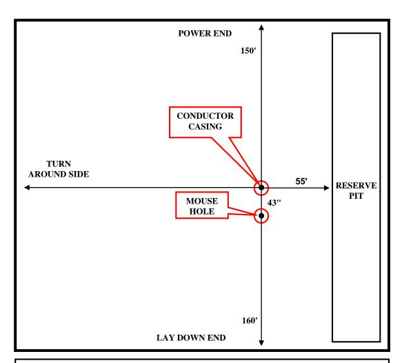
**Note:** <u>All</u> measurements are from the center of the conductor casing. The mouse hole is 43" from the center of the conductor casing  $w/0^{\circ}$  slope (angle). This rig has a top drive so the mouse hole should be a minimum of 75' deep (from ground level) with casing or liner with a minimum ID of 10". The reserve pit is a minimum of 55' from the center of conductor casing.
