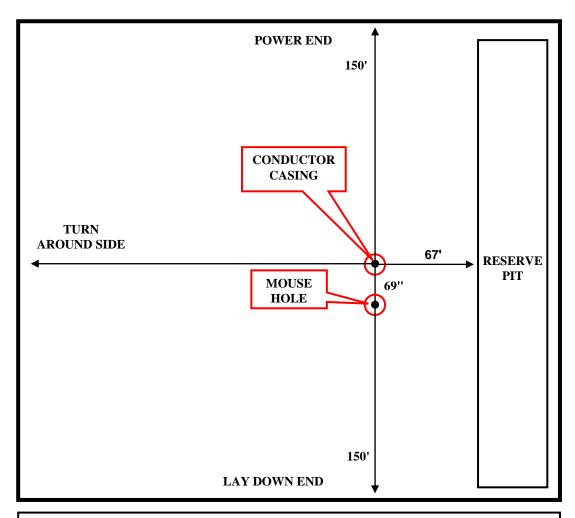
**Note:** <u>All</u> measurements are from the center of the conductor casing. The mouse hole is 69" from the center of the conductor casing w/0° slope (angle). This rig has a top drive so the mouse hole should be a minimum of 75' deep (from ground level) with casing or liner with a minimum ID of 10". The reserve pit is a minimum of 67' from the center of conductor casing.
