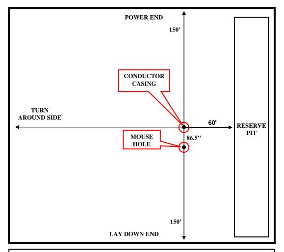
**Note:** <u>All</u> measurements are from the center of the conductor casing. The mouse hole is 86.5" from the center of the conductor casing  $w/0^{\circ}$  slope (Angle). This rig has a top drive so the mouse hole should be a minimum of 75' deep (from ground level) with casing or liner with a minimum ID of 10". The reserve pit is a minimum of 60' from the center of conductor casing.
